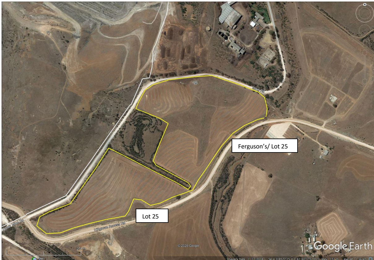
Figure 6 GE Image November 2018, SEB Offset Commencement on Ferguson's & Lot 25. Note the red/brown strips, which have been pre-stripped, ripped and direct seeded with native seed mixes.
